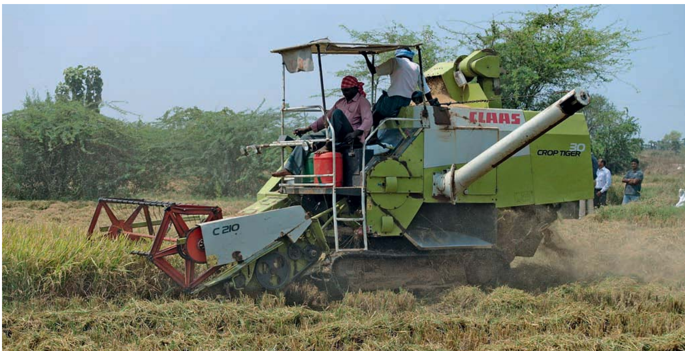
Model Crop Tiger in India, developed by Claas. It was originally designed for the rice harvest. Thanks to further developments, it now has the ability to tackle grain as well.
